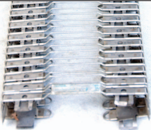
This piece of the B-52 was found near the crash site and identified as a Flexible Ammunition Chute.
