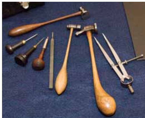
Top: An ornate revolver after completion by J.J. Roberts. Above left: The Lindsay air driven palm tool. Above center: Traditional tools – hand graters and specialized hammers for “chasing” the hand graters. Round handled graters are for pushing while the straight/no handle graver is for chasing. Above right: Finished script letters.
