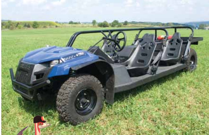
Above: The enhanced EMU (Electric Mine Utility Vehicle), developed at Pillar Innovations is built on a Polaris ATV platform with major modifications and custom features for rigorous mining tasks.
