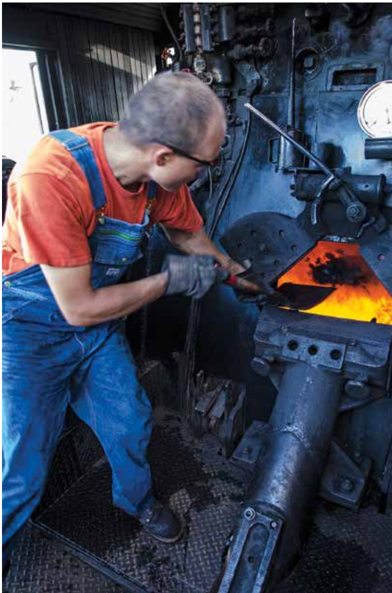
Fireman, Steven Diehl shovels coal into the firebox to maintain steam pressure at 195 psi.
