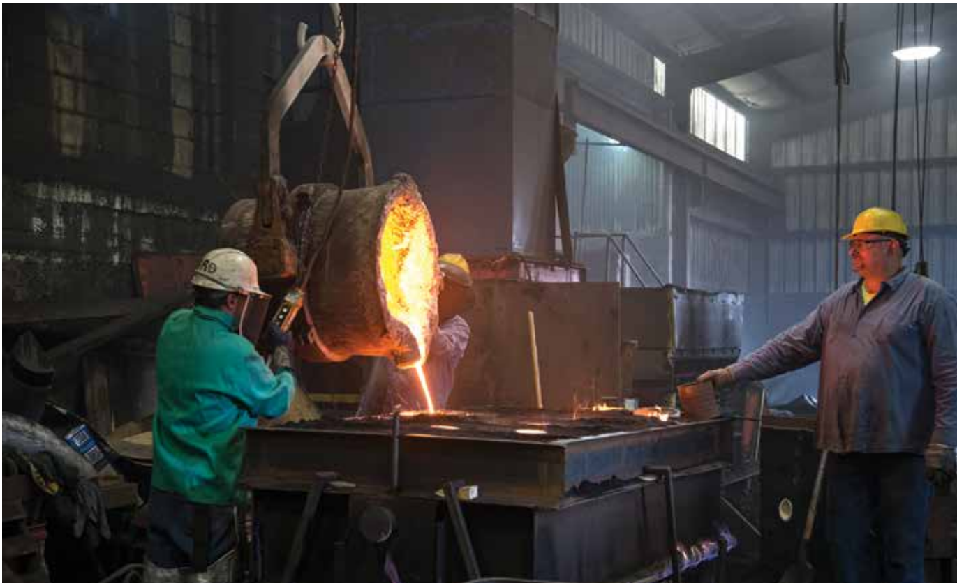
Top Photo: Scraping the Slag off the ladle. The Slag is the impurities that float in the molten iron.
