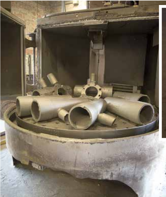
Above: The Shot blaster after the castings shake out from the mold but before the grinders remove the gates and riser.
