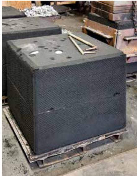
Top Left: Pin Lift Machine Molding.
