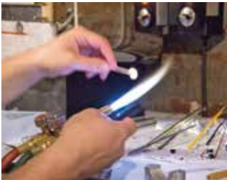
Producing the gather after the cane has been heated.
