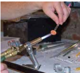
Color is placed on the disk—gravity pulls the color to the center of the bead.
