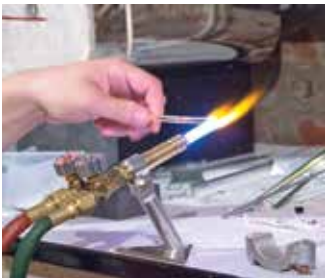
The "soft glass" cane is heated in the flame.
