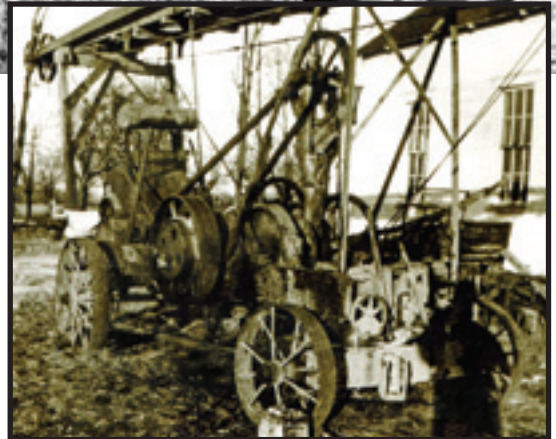
About 1932; Aubrey Brenneman and son, John, on a homemade tractor made from a Model T Ford. The front tires are solid rubber.
