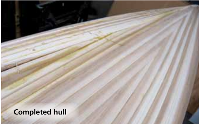
\frac{3}{4} " x \frac{1}{4} " strips of red cedar placed over the strong back to form the hull
