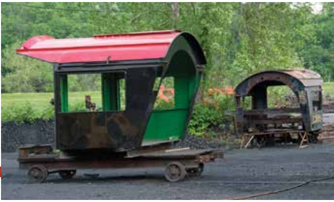
The new cab for #1309, almost ready for installation, sits alongside the old #1309 cab.
